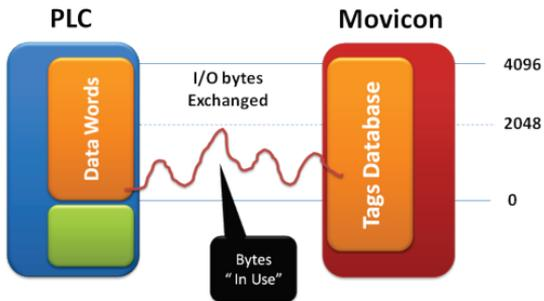
*This chart shows a project connecting 4096 I/O bytes simultaneously, but not more than 2048 Bytes actually go into use. Therefore a license with 2048 I/O bytes is needed.*
