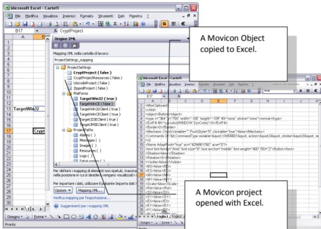
Each object's XML structure can be accessed directly through the XML Explorer window using the Movicon editor to modify its properties textually.
