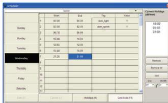
The Timetable mode allows you to select the exact hour and minute, the variable associated to the command and the assigned value.
