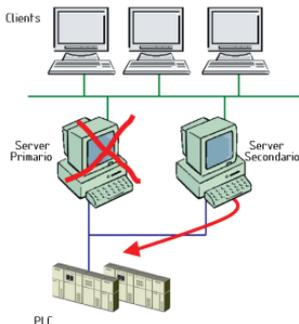
*Simple redundancy architecture*
