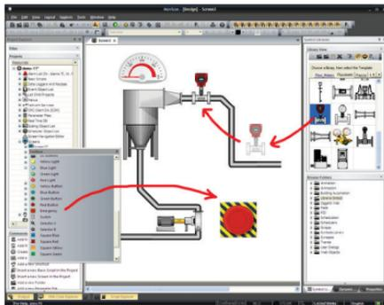
*The object-oriented programming uses the drag&drop techniques to insert symbols and objects on screen as well as to assign tags. Configurations are done using the property windows.*
