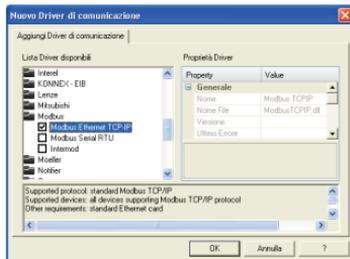
The drivers automatically optimize communications by exchanging only those tags effectively in-use in the project with devices. The features of the different driver functionalities are described below.
