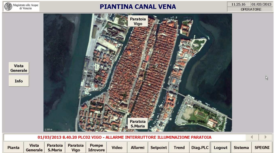
3. The Movicon supervisor of the BabyMOSE system shows the geomap of the Canal Vena where the floodgates have been installed: the Vigo and Santa Maria floodgates.
