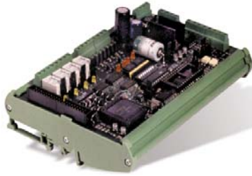
I/O modules distributed on buses made by PICOdata
