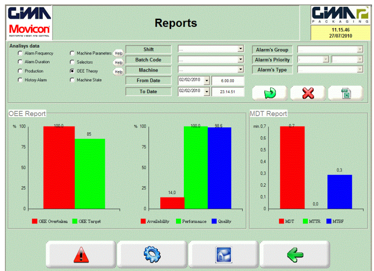
The main performance indexes (OEE) presentation. All data managed by the supervisor can be accessed via Web Client.
