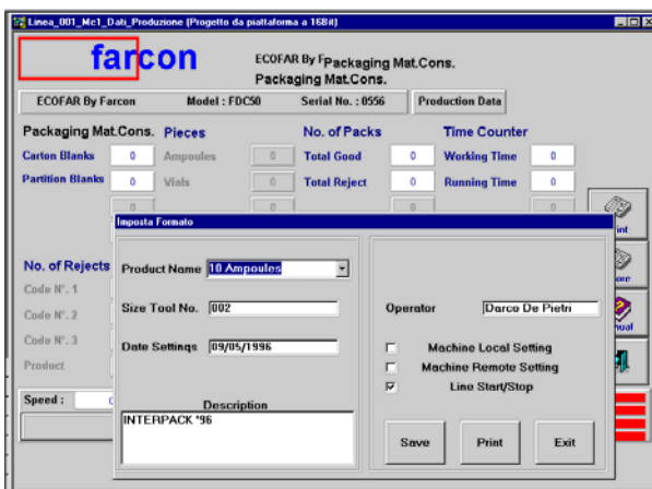
Parameters are set through dialog windows that guide the operator in configuring the machine production process.
