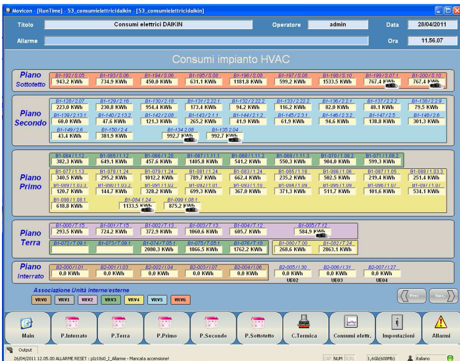
Figure 4 – Screen displaying HVAC system consumptions
