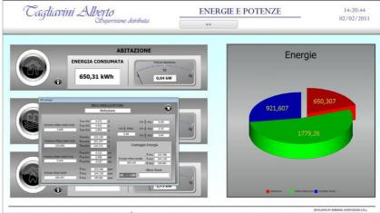
water temperatures, chlorine concentrations, PH and acidity as well as the working status and running of the heated pool facilities, such as temperatures, central heating (boiler, water pumps and radiators), all process data deriving from the photovoltaic systems with regular energy consumption analysis of the whole structure, all of which is performed through the touch screen interface.
