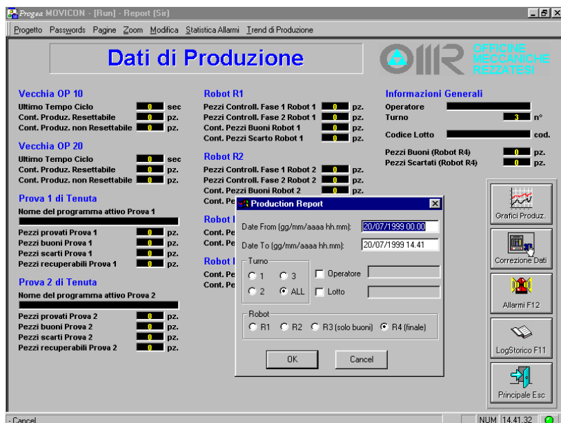
This page reports production data in realtime. The operator can use this page to get statistical production analysis by specifying the required information. Movicon creates statistic reports and production chart graphics.
