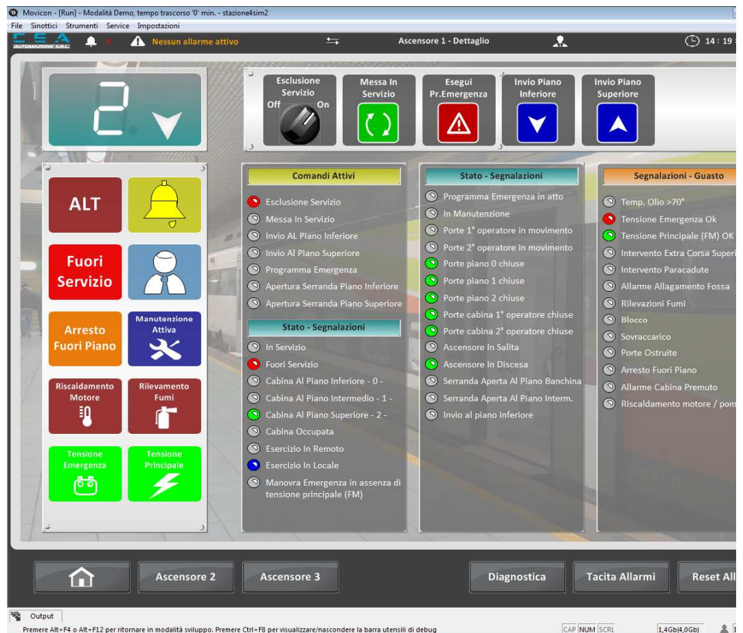
4. A detailed Movicon screen page of lift 1 showing all the settable parameters
