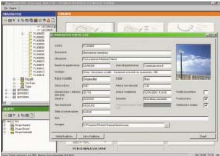
Figure 1 – This is an example of screens used for reporting data of electrical light points (supports, man holes, drains, lighthouses, etc), associated with a number with all information describing the situation of each object.
