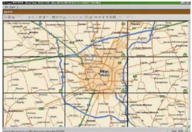
Figure 2 – This shows interaction between animated map, anagrphical data and telecontrol. A green light, on the bottom right of each square on the map, means that there have been no alarm occurrences in that zone as yet.
