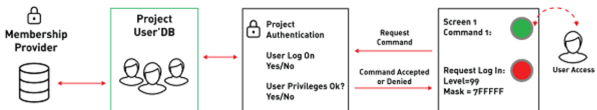
This is an example of command access protection and the authentication and permission process
